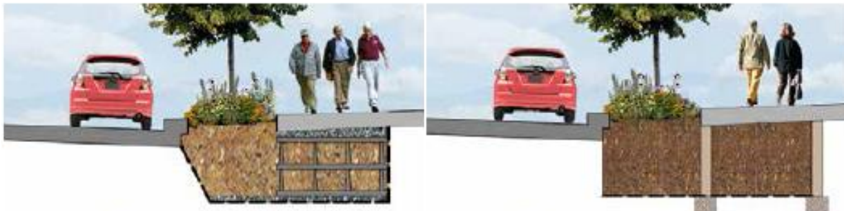
Figure 2-3 Stormwater tree well filter conceptual examples: modular suspended pavement system (left), column suspended pavement system (right). (Courtesy of Philadelphia Water Department)
